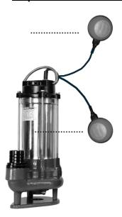
The installer should pay attention to the size of the chamber the pump is installed and the expected inflow rate. Undersized pump chambers result in pump cycling and increased risk of overheating
